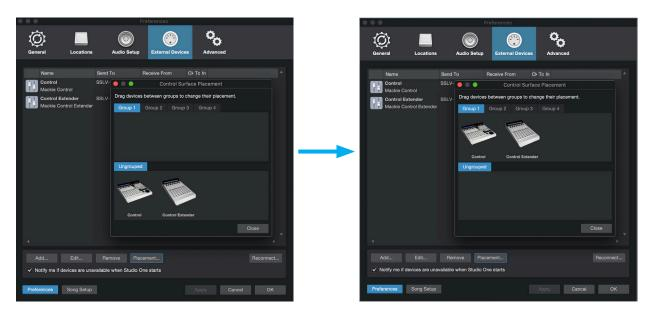
STEP 7 : Go to Control Surface Placement setup and click and drag the Mackie Control and Mackie Control Extender(s) and move them up into Group 1.
