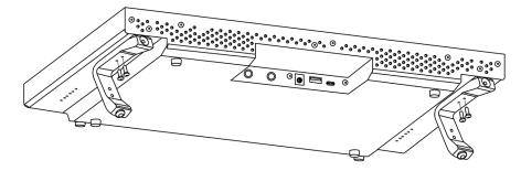
UF8 has been designed to be used with or without the included screw-in stands, depending on your preference. Attaching the included screw-in stands has the added benefit of angling the unit towards you. Three different fixing positions (the holes are arranged in pairs) allow you to choose an angle that is best for your setup. Use 2 screws per stand. **Please be careful not to over-tighten to avoid stripping the screw threads**. For those with a torque measuring device, tighten to 0.5 Nm.
