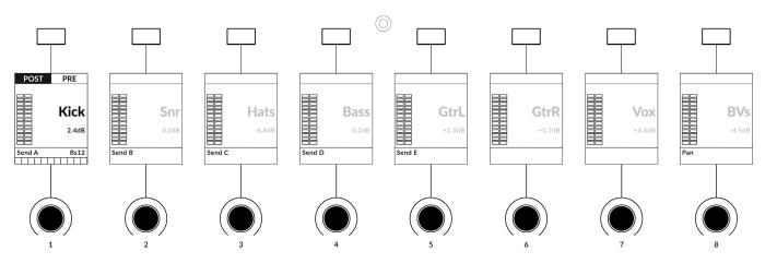
STEP 3: Use V-Pots 1-5 to control Sends A-E and V-Pot 8 to control Pan.
