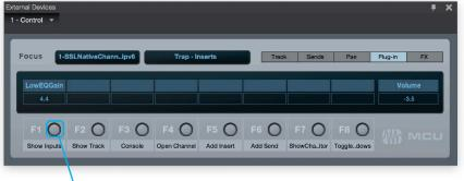
Right-click on the button and click 'Assign Command...' to change the function of any of the F keys.
