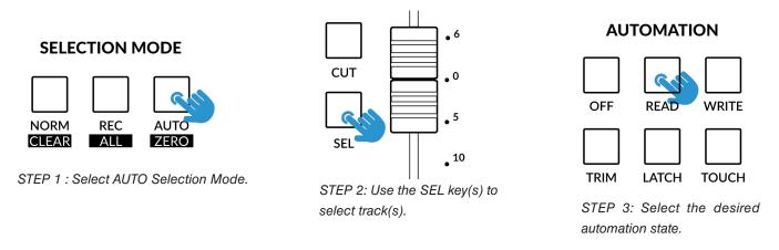
Multiple tracks can be selected at once using the Shift/All (contiguous) and Opt/Alt modifier keys (all). Non-contiguous selections can be achieved pressing and holding the first SEL key and then pressing subsequent SEL keys.
