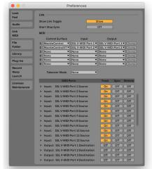
STEP 5 : Add a MackieControl and configure for SSL V-MIDI Port 1 on Input and Output
