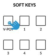
STEP 1 : Press V-POT a second time to toggle Soft Keys keys into Send Mute Mode.
