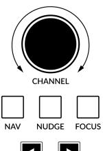
By default, the **CHANNEL** encoder is used to move your DAW tracks across the UF8 surface, in increments of 1 channel at a time. If you find yourself in **NAV** or **FOCUS** modes, simply push the **CHANNEL** encoder to return to **CHANNEL** mode.
